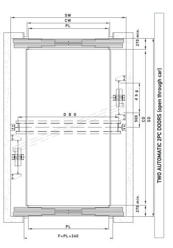
Dimensions of Hydraulic Bed Lifts Indirect Single Ram Side Acting (HADI 1:2) or Direct Single Ram Side Acting (HAD 1:1) **2-Panel Telescopic Opening Automatic Doors**
